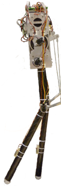
Figure A.8: Photograph of the bipedal robot—The robot design corresponds to the model described in Section A.4.1.
